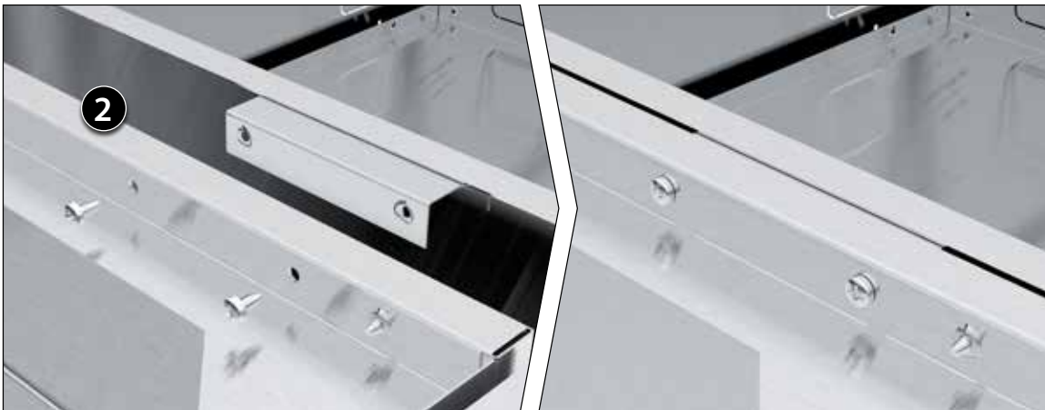
Latch the top L-Bracket from the adjoining cabinet over the cabinet and secure with screws.
